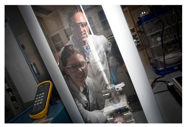
National Energy Technology Laboratory researchers Elliot Roth and Megan Macala sonicate coal-based materials to enhance particle separation and the extraction of rare earth elements.
